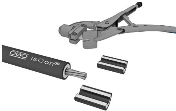
Fig. 12 Laying the copper core bare
